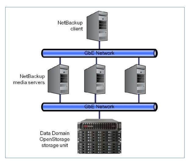
Figure 6: Segregated network for Data Domain traffic
